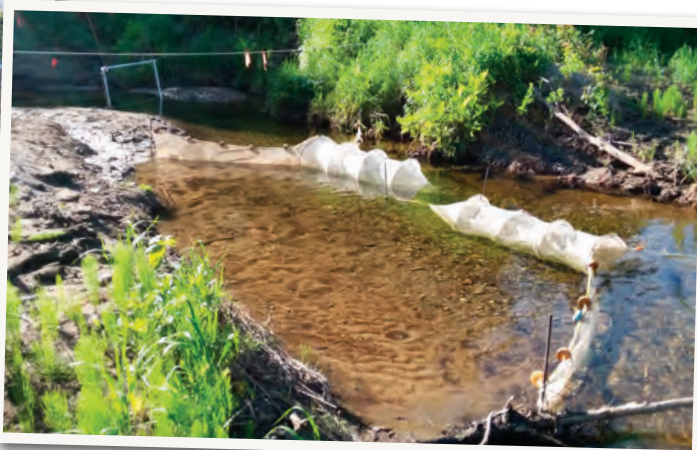
These fyke nets were used to capture wild brook trout migrating into and out of Loomis Valley Brook as part of a study to learn more about the migratory behavior of brook trout in the Dead Diamond watershed.
