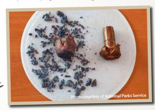
A recovered .270 caliber copper jacket lead-core bullet (left) is heavily fragmented compared to the solid copper bullet (right) that retained its original shape upon impact.
