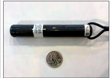
Above: An acoustic receiver listening for pings at the Block Island Wind Farm.
