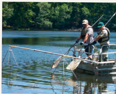
Fisheries biologist capture bass and other warmwater fish with an electrofishing boat.
